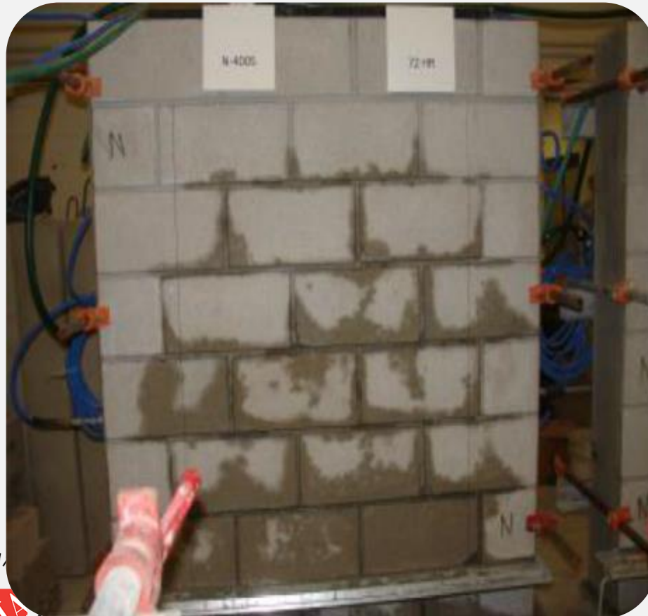
Wind Driven Rain Test E514 after 72 hours Untreated CMU/Mortar.
