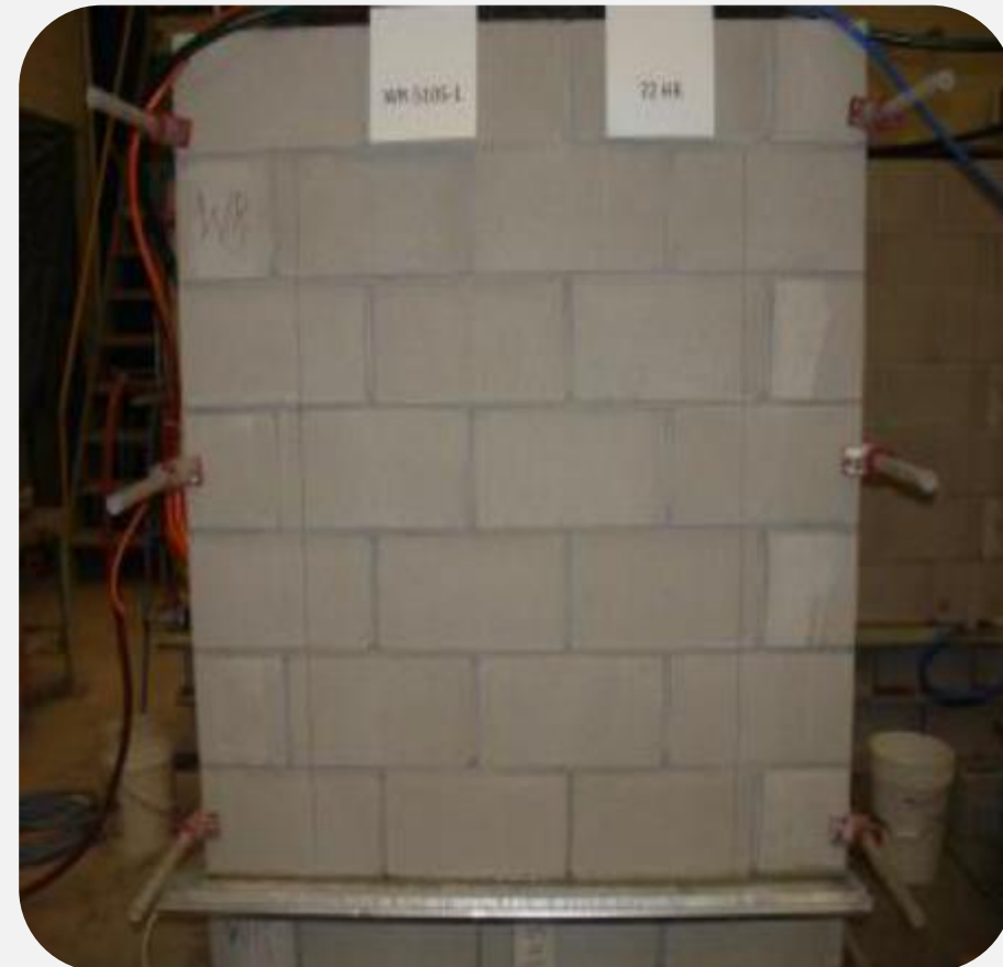
Wind Driven Rain Test E514 after 72 hours CMU/Mortars with Integral Water Repellent
